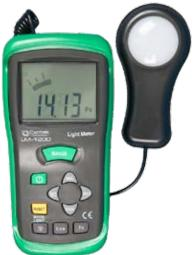
The Light Meter LM-1200 is a precision instrument used to measure illuminance (lux, footcandle) in the field. It meets the CIE photopic spectral response specification ans is fully cosine corrected for the angular incidence of light. The illuminance meter is compact, rugged and easy to handle. The light sensitive component used in the meter is a very stable, long-life silicon photo diode and spectral response filter.
