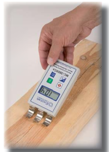
Measuring depth 100 mm, - Can detect moisture cavities in a wooden beam
