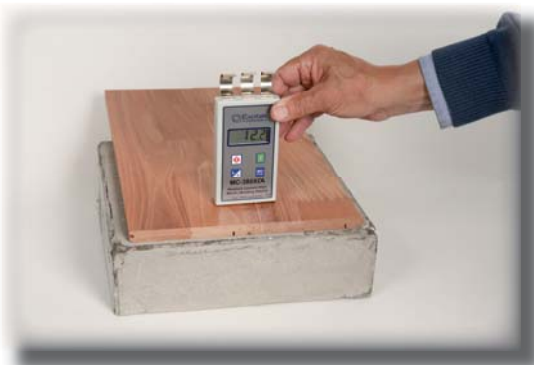
Measuring depth 10 mm - Measures only the wooden floor
